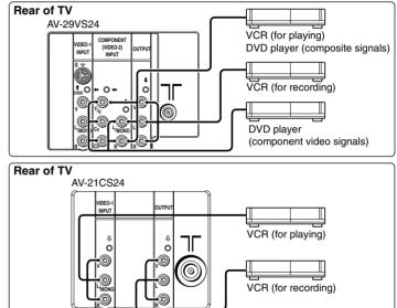
When you use VIDEO-1 INPUT, you should choose to connect S-VIDEO or video input. If S-VIDEO connector and video input are connected at the same time, no picture displays on the screen and the message "PLEASE DISCONNECT VIDEO-1 CABLE!" appears. In this case, you should disconnect either S-VIDEO or video input.
